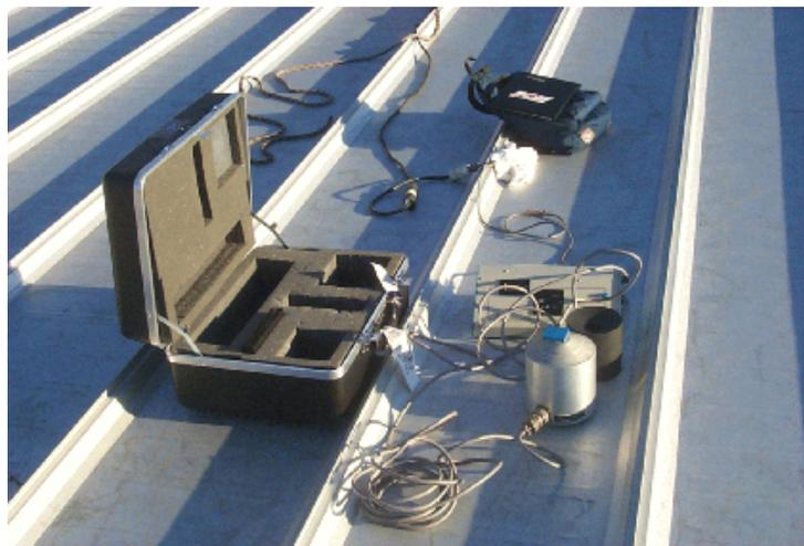
**Figure 1** Devices and Services Company reflectometer
